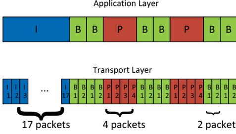
Fig. 1. Transmission of data in application and transport layer
