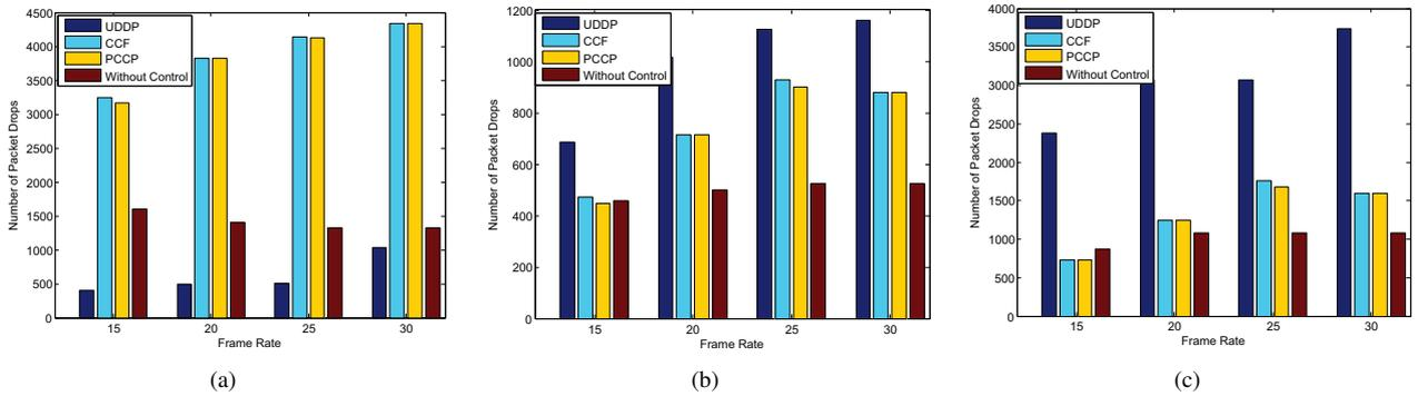
Fig. 4. Average number of packet loss for a) I-packets, b) P-packets, c) B-packets
