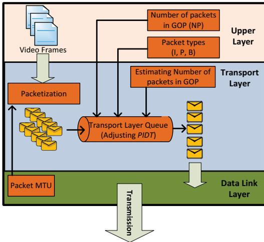
Fig. 2. Cross layer architecture of the proposed protocol
